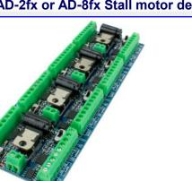
These make wiring easy and give fantastic versatility in control - they also provide added on-board switching AND feedback or computer IO ability. Connect to the track or accessory power bus—or for DC users, use a 12~15v regulated DC wall plug supply to power them.
