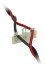
**Step 4 - Insert the bare area of the power bus into the loops.** When that is done, you can close the loops again. Solder the bus wires to the tag loops. The image (left) show what we mean here. Neat and tidy, isn't it?
