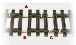
2) **Prepare the track or turnout**. Decide where the dropper will go. If needed, remove the web from between two sleepers, exposing the bottom of the rail. Rail oxidises even when new (A), so clean it well (B) using a file or fibreglass brush.
