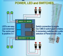
Power Connections (only one power input powers all outputs)
