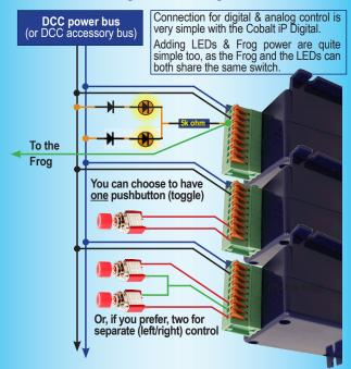
Even when LEDs or pushbutton switches have been added, you will still have one SPDT switch free and available for signals, interlocking or any other purpose that you choose.
