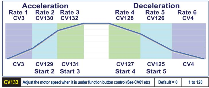
Adjusting this CV will let you set the motor run speed OR the operating voltage of a device that is connected to the DECODER MOTOR DRIVE CIRCUIT if you are controlling it via a function button. (Please refer to CV61 and other information on the CV61 page for detailed information on how to initiate button control).
