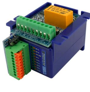
One of the products we seem to have "left in the shade" with our growing focus on "DCC onboard" point motors is the great value AD-1 High power DCC Accessory decoder.
