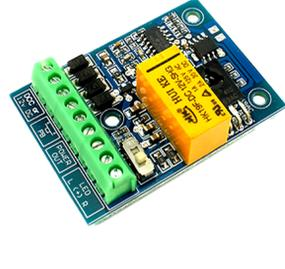
To this high power ability we added DC or DCC power capability, push button switch control and direct LED connections (with no resistor needed). Altogether, it's great value!
