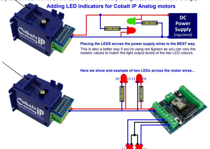
Of course, if you use DCCconcepts AD-2fx or AD-8fx decoders... With EITHER Cobalt iP Analog or Cobalt  $\Omega$  Omega - you have the choice of adding the LEDS to the decoder (or you can use decoder outputs for other things like computer I.O. or light-signal control)
