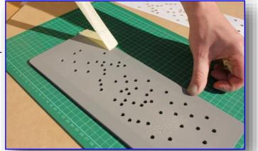
(Because the holes in the support panel and diagram match, the pencil end-tapers guide them together and this results in accurate registration between the panel parts.)
