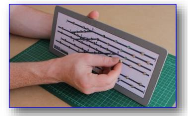
Additional switches and LEDs can also be bought from DCCconcepts. Both the switches and LEDs have 1/4" threaded mounts. The ideal tool to do them up is a small tube-type nut wrench or spanner - however if you are careful, pliers will do.
