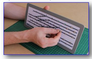
Additional switches and LEDs can also be bought from DCCconcepts. Both the switches and LEDs have 1/4" threaded mounts. The ideal tool to do them up is a small tube-type nut wrench or spanner - however if you are careful, pliers will do.
