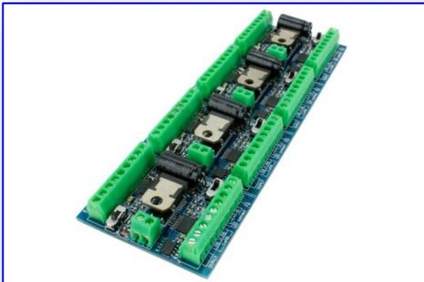
These make wiring easy and give fantastic versatility in control - they also provide added on-board switching AND feedback or computer IO ability. Connect to the track or accessory power bus—or for DC users, use a 12~15v regulated DC wall plug supply to power them.
