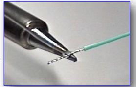
Where there's a fine bead to be sweated to the edge of a sheet, where parts are to be "laminated" as in inner & outer halves of a coupling rod or where an overlay has to be allied to a tender side etc.
