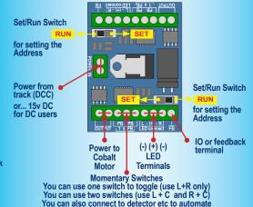
With all AD-2fx wiring able to be done by screw connector and with spring connectors on all Cobalt Classic, Cobalt iP & Cobalt \O Omega motors plus clear instructions printed onto the PCB... wiring just couldn't get any easier.
