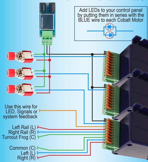
Cobalt Classic  $\Omega$  has a "Voltage Range Switch" on the PCB, This gives a choice of 6~12 or 12~18v DC & all you need to do is change the switch so that it matches your Power supply voltage or Accessory decoder output.
