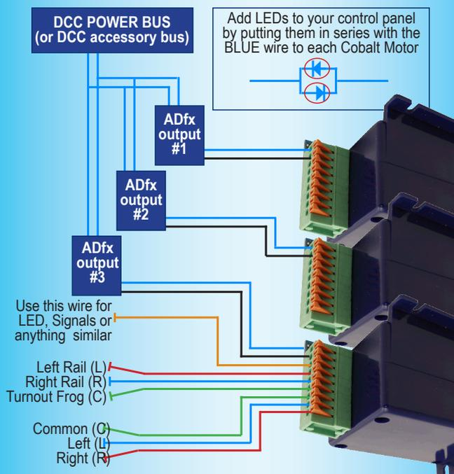
DCCconcepts AD2fx and AD8fx Decoders have enough power to change several Cobalt plus new features including optional 1 or 2 button control AND direct computer IO or feedback. They work well with DCC & DC too
