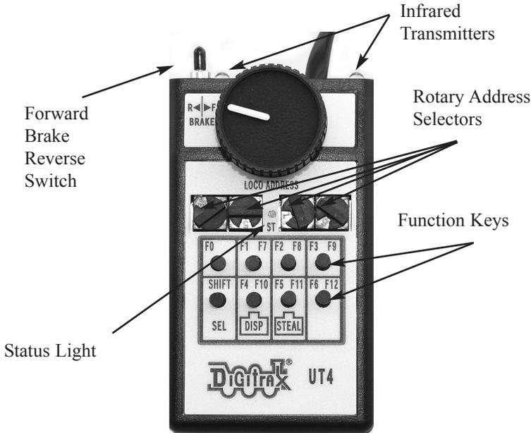
**Note:** The UT4 is a utility throttle that is primarily intended for locomotive control. It cannot program decoders, throw turnouts, or turn track power on or off.
