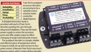
ports can be programmed in one go by selecting the lowest numbered address and changing it on a DCC handset with the learn button switched on.
