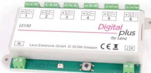
clearly labelled. Addressing can be done in two ways - block addressing for all six outputs in one go or individual addressing of each port on the decoder. This makes this a highly flexible piece of kit with great advantages.
