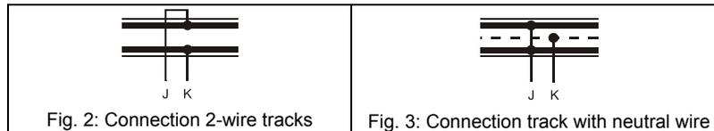
Fig. 2: Connection 2-wire tracks
