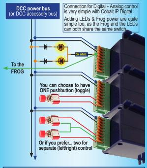
Even when LEDs or Pushbutton switches have been added you will still have one SPDT switch free and available for signals, interlocking or any other purpose that you choose.
