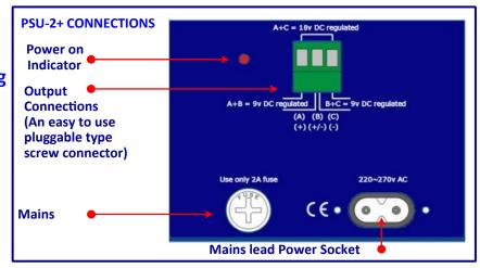
PSU 2+ is a totally self-contained, mains powered, stable dual output power supply that can power a layout full of Cobalt point motors at 9 volts DC AND at the same time, it can also be wired to give a stable 5 amp 18v regulated DC power supply.
