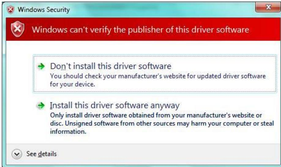
The base drivers are fully compatible with Windows7, and those supplied on the CD are the latest drivers. To make them SPROG NANO specific, the .inf files are edited which, unfortunately, causes this dialogue to appear.
