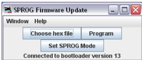
First the old firmware will be erased, and then the new firmware will be written. Progress is reported in the status line of the window. If the Console is still open, you will also see the messages flowing between the computer and the SPROG Nano.
