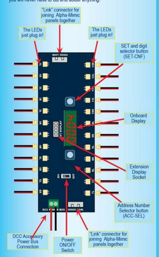
Your Alpha Mimic panel can be supplied with Red, Green or dual colour Red+ Green LEDs and it includes the following: \* 1x Alpha Mimic PCB \* 1x Alpha Mimic interconnector lead \* 24x Alpha Mimic LEDS \* Instructions
