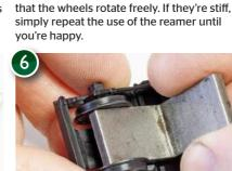
Another check to make is the back-to-back measurement - that is, the distance between the inner faces of the wheels. For 'OO', this should be 14.5mm, whereas finescale 'OO' and 'EM/P4' have their own specifications
