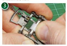
A choice of reamers is supplied with different Test-fit your new wheelsets, checking that the nylon 'handles' to suit different bogies or underframes. Gripping the axleboxes prevents the bogie sides being pushed apart while the
