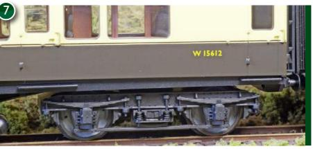
Refit the bogies and test the model on your layout, looking out for how it runs over points and crossovers. These Gibson wheels have made a massive difference to looks and performance. although the centres require painting
