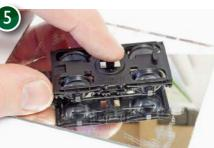
It helps to check that the new wheels and axles are installed correctly by placing them on to a sheet of glass. All four flanges should be in contact with the glass, otherwise one of
