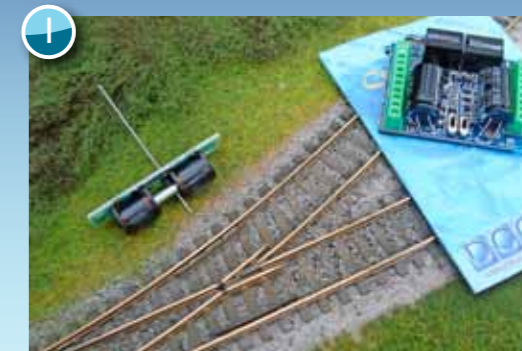
The basic ADS-2fx unit will operate four solenoid point motors.
