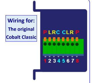
Cobalt Classic wiring. Input voltage must be 9 to 12v DC. Please use a regulated DC power supply & NOT the 12v uncontrolled output of a train-set transformer which will be closer to 16 volts when under light loads.
