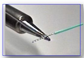
It is also sometimes very helpful to pre-tin tiny parts such as lamp irons. Then, if the footplate is tinned as well, all that is required is a little flux and a quick application of the iron and the job is done with no need at all for any additional solder. (Much neater than adding solder while its in place)
