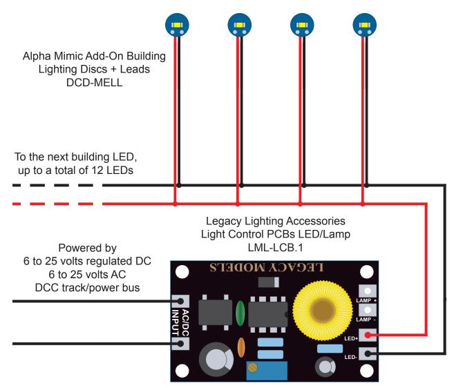
Adjust the overall brightness using a small screwdriver on the brass screw.
