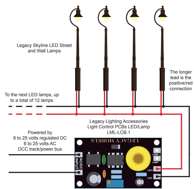
Adjust the overall brightness using a small screwdriver on the brass screw.
