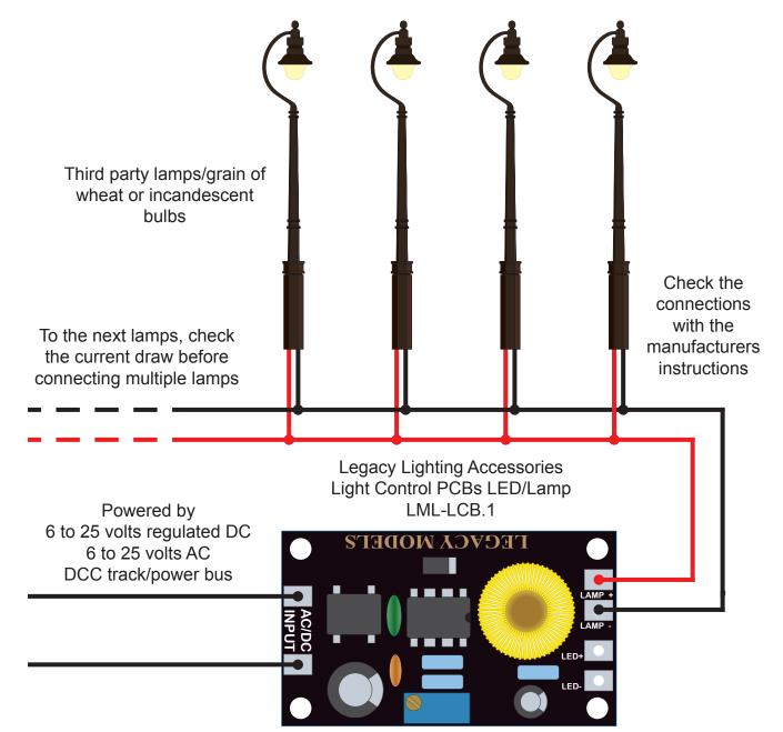
Adjust the overall brightness using a small screwdriver on the brass screw.
