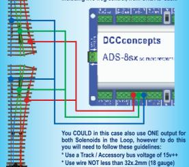
You COULD in this case also use ONE output for both Solenoids in the Loop, however to do this you will need to follow these guidelines: \* Use a Track / Accessory bus voltage of 15v++ \* Use wire NOT less than 32x.2mm (18 gauge) \* Keep the wires short as possible AND keep the wires the SAME length to each of the solend (Also try using more efficent solenoids. Examples are Gaugemaster PM10 and PM20. They are 6 ohms rather than 4 ohms. This assists efficient operation)
