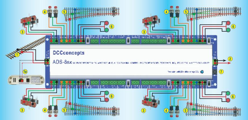
There are EIGHT outputs on the AD-S8sx. Rather than create a totally confusing drawing, we have used only four sets of connections here. The other four connections are of course, identical in layout.
