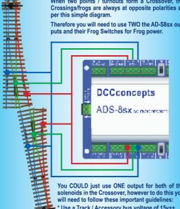
You COULD just use ONE output for both of the solenoids in the Crossover, however to do this you will need to follow these important guidelines \* Use a Track / Accessory bus voltage of 15v++ \* Use wire NOT less than 32x.2mm (18 gauge) \* Keep the wires short as possible AND keep the wires the SAME length to each of the solenoids.
