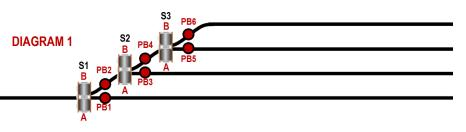
Operation is more complex too as to reach the top siding you would need to press 3 switches... PB2, PB4 and PB6.
