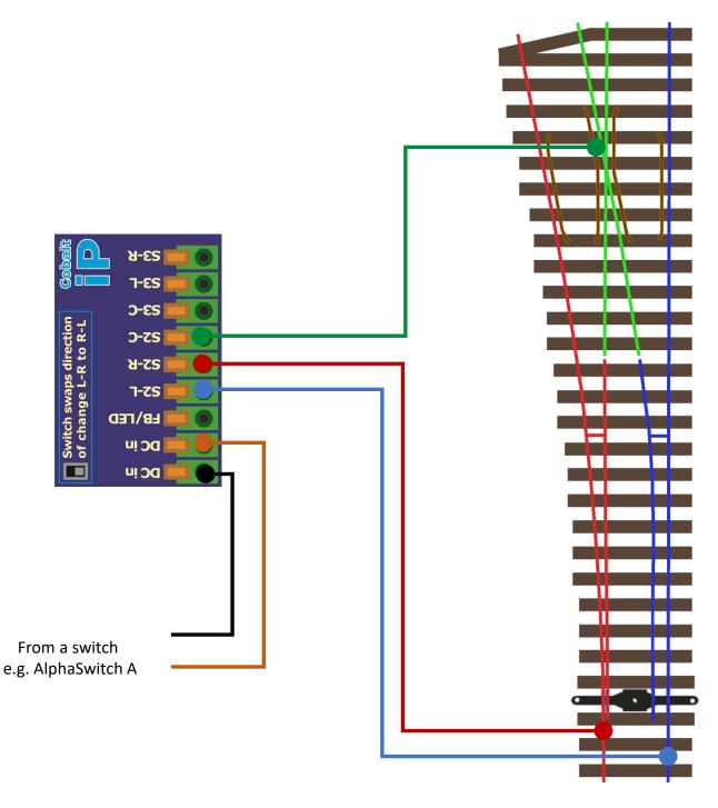
Orientation of the Cobalt will affect the wiring. If the point frog polarity is incorrect, swap **S2-L** and **S2-R**
