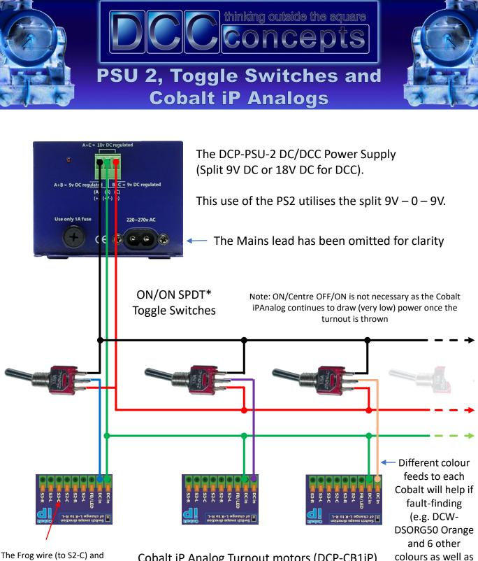
The Frog wire (to S2-C) and Dropper wires from track (to S2-L & S2-R) have been omitted for clarity
