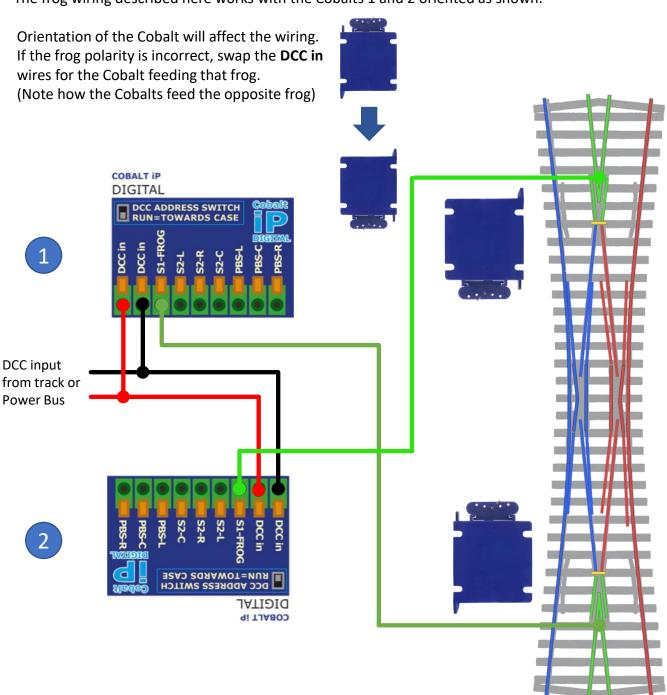
Note: The wiring is different if using an Accessory Bus where connections S2-L and S2-R are used to take the power feed from the Track Bus or track itself, and then feed the frog via S2-C.
