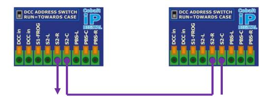
Tip: Use this switching logic to feed a buzzer or an LED. Use S2-L if the Cobalt is oriented the other way.
