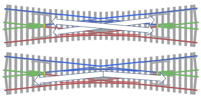
However, on a 2-rail electric model railway, in order to achieve correct frog polarity there are three turnout position scenarios to do this.
