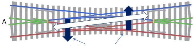
Tiebar (and so turnout motor) positions
