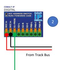
The orientation of the Cobalt will affect the wiring. If a turnout frog shorts, swap its Cobalt's **DCC in** wires over. This doesn't affect the command to the Cobalt i.e. STRAIGHT is still ahead and RIGHT is still right.
