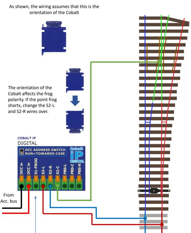
The frog needs power taken from the track or track bus. Therefore the connection "S1-Frog" can not be used as it takes its feed from the accessory bus not the track.
