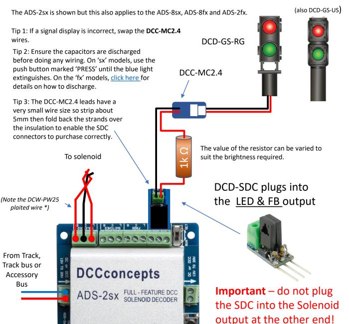
\*In addition to making wiring neat and tidy, the plaiting of the 3 wires greatly reduces induction within the wire, increasing power delivery and, because it reduces the high voltage spike that happens each time the solenoid coil power is released, it also helps to extend switch life and increase reliability.
