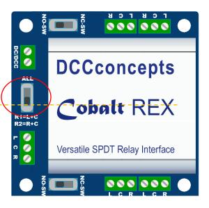
Connecting the devices that you want REX to control uses the 3-terminal blocks close to each relay. Each 3-terminal block is effectively an SPDT switch. Switch connections are all set up as Left - Common - Right.
