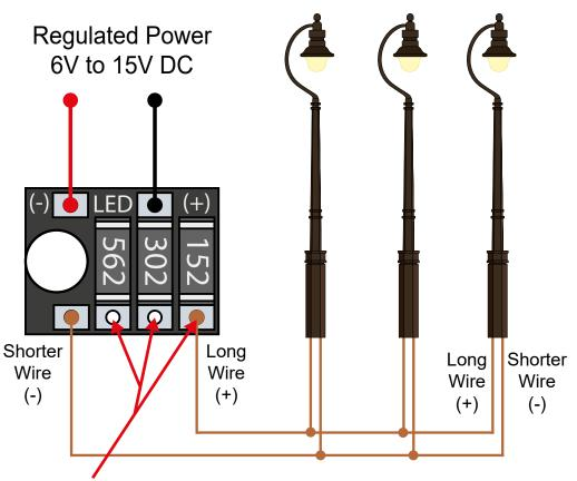
Connect the long cable to the resistor value you want for the brightness of the lamps. This will vary depending on the power supply value you use.
