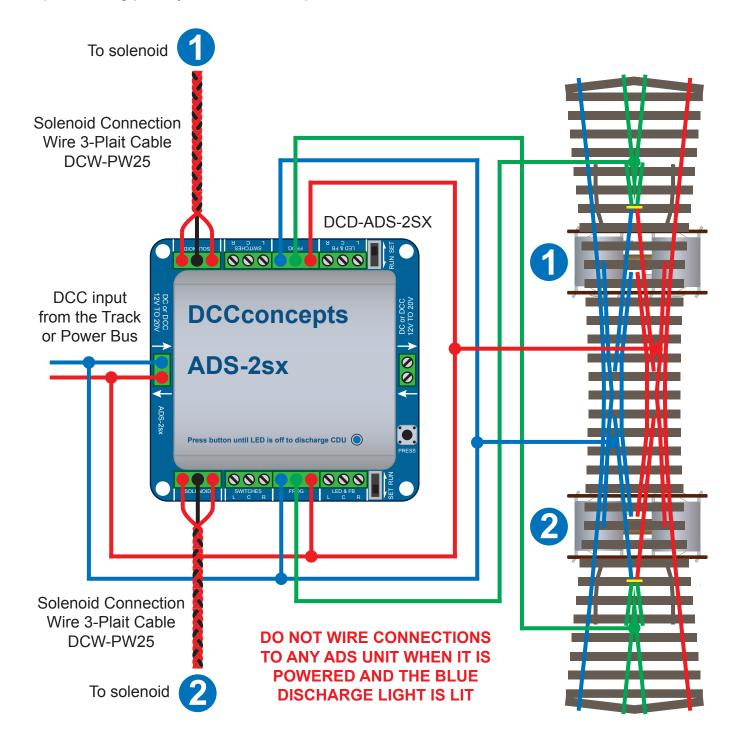
In addition to making wiring neat and tidy, the plaiting of the 3 wires greatly reduces induction within the wire, increasing power delivery. This is because it reduces the high voltage spike that happens each time the solenoid coil power is released. It also help to extend the switch life and increase the reliability.
