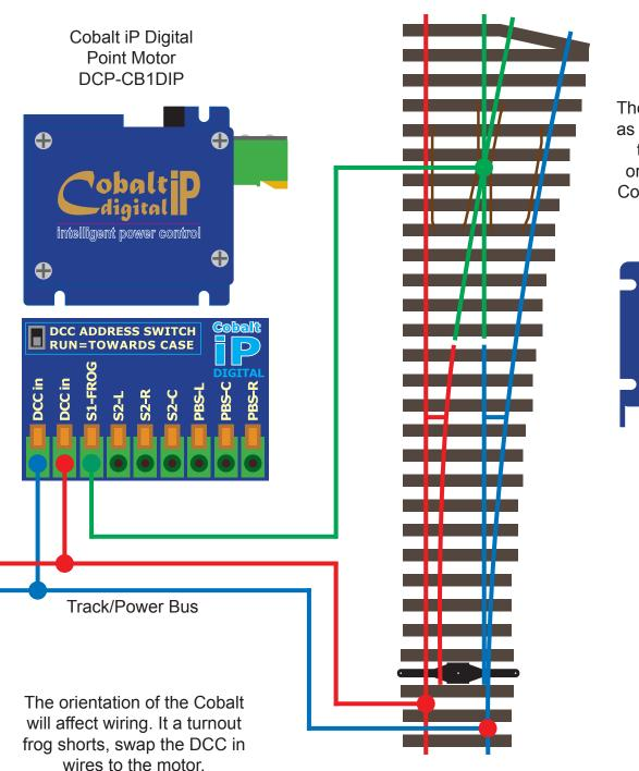
The wiring diagram as shown assumes that this is the orientation of the Cobalt point motor.
