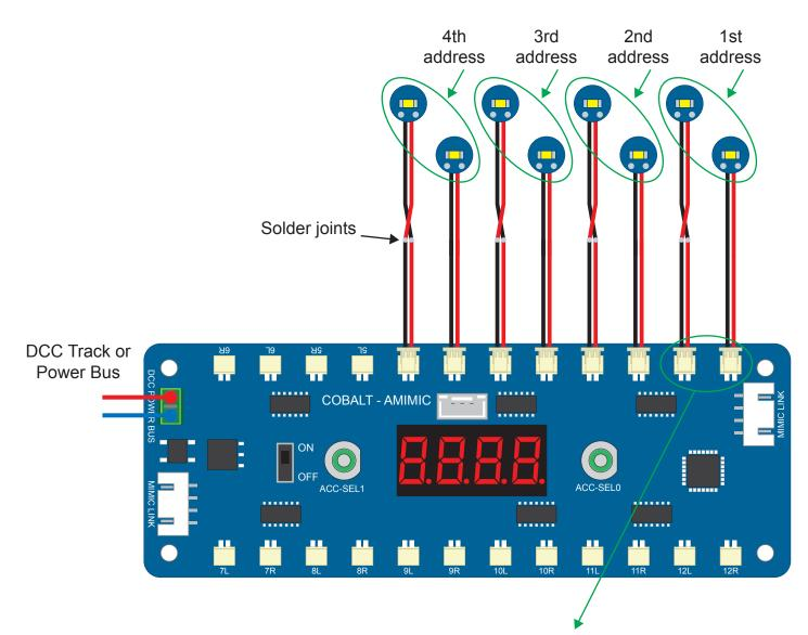
If the LEDs are on when they should be off, swap the two connections in the L and R sockets on the Alpha Mimic board.
