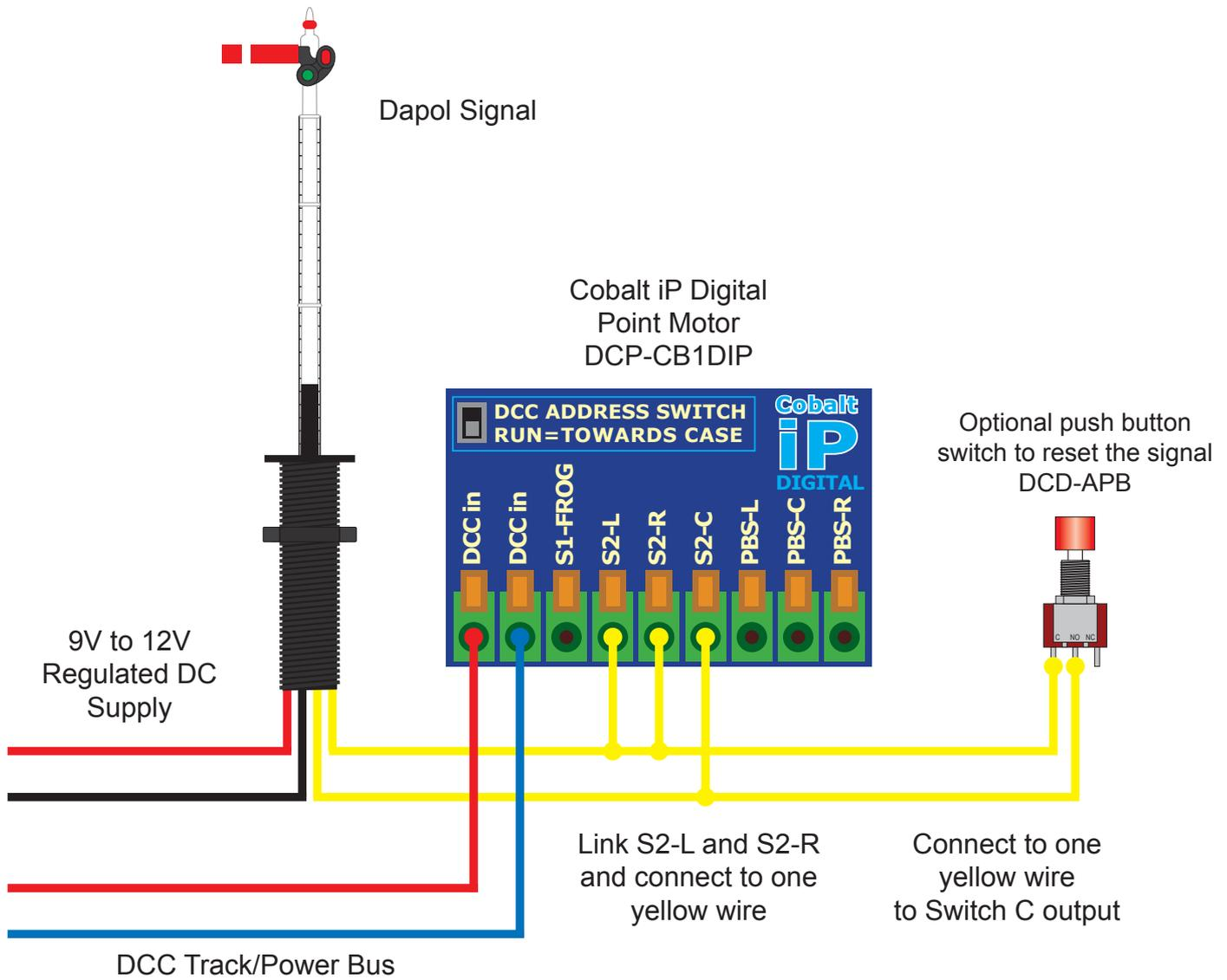
The Dapol signal mechanism has an unfortunate habit of getting out of sync with the point motor. The push button switch would be used to reset/re-sync the signal with the motor.
