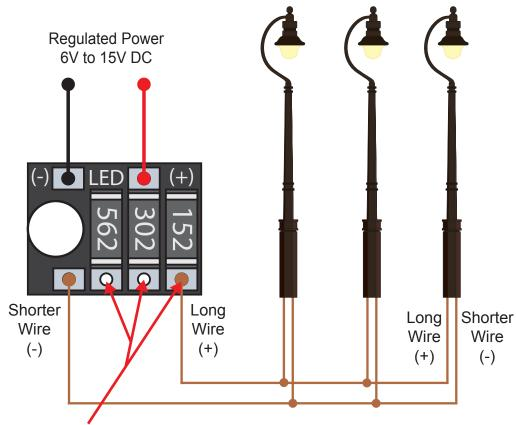
Connect the long cable to the resistor value you want for the brightness of the lamps. This will vary depending on the power supply value you use. The longer wire from each lamp is the positive connection, connect up the lamps in parallel as shown above. Each resistor board can connect up to 3 separate lamps.
