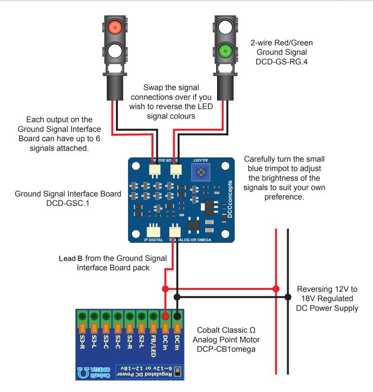
NOTE - ONLY connect one point motor connection lead at any one time or you may damage the circuit board.
