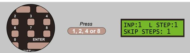
A **SKIP** command will skip over the designated number of steps if the selected input is in the designated state at the time the **SKIP** is executed. A **SKIP** command does not rely on a CHANGE of state of the subject input.
