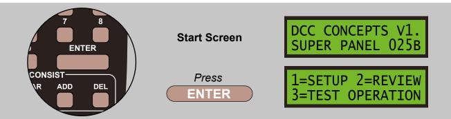
Select 1=SETUP by pressing 1, and then 2=SET CONFIG by pressing 2:
