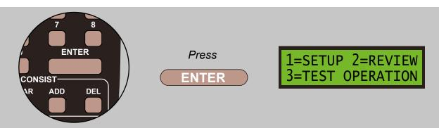
At each menu level, there may be functions available that are not visible on the two-line screen. Press the **DEC** key to scroll down one line, moves the text up one line, or press the **INC** key to scroll up one line, moves the text down one line. You can also use **SPEED** control wheel to move the text up or down a line:
