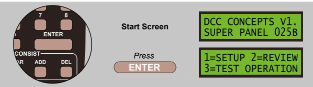
Select 1=SETUP by pressing 1, and then 2=SET CONFIG by pressing 2:
