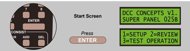
Select **1=SETUP** by pressing **1**, and then **1=SET INPUT** by pressing **1**:
