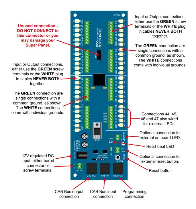
DCCconcepts use the 2 pin JST sockets extensively on its products. These are usually used to connecting Mimic LEDs to a device/circuit board.
