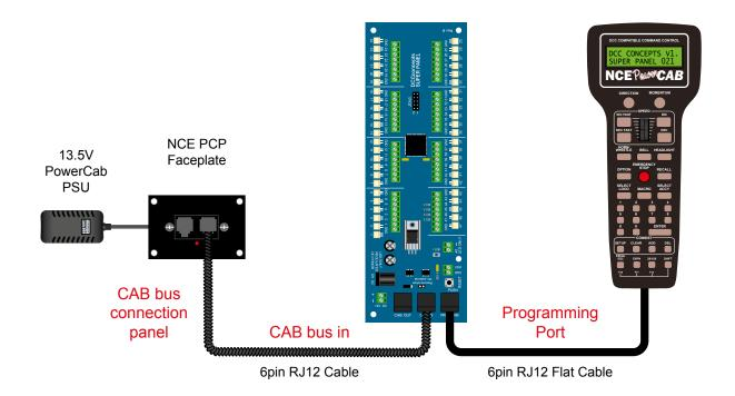
The Super Panel can be programmed whist connected to your CAB bus. Depending on what you are programming we suggest removing the CAB OUT connector whist performing this task.
