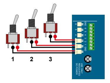
If you are using the supplied **RED** and **BLACK** 2 pin cables with the JST connection, the **SIGNAL** and **GROUND** are included in the same connector block.
