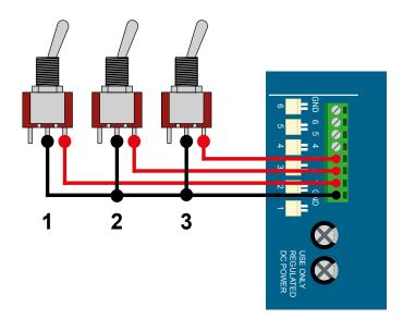
When connecting a device to the Super Panel, if you use the **GREEN** screw terminals, the Super Panel has a set of **COMMON GROUND** connections throughout the board.
