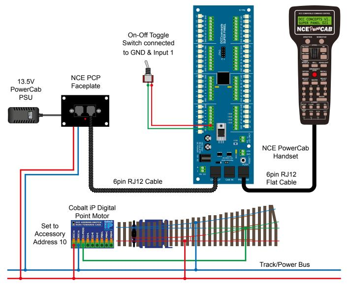
The **ON-OFF** toggle switch is connected with the centre common to one of the Super Panel ground connections, and the switched connection to Input 1 on the Super Panel.
