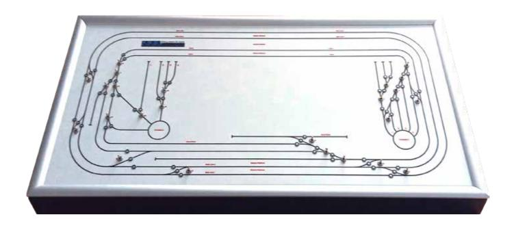
This control panel included multiple Alpha Encoder Units, Alpha Mimics, box size 5 and controlling 28 DCC accessory address.
