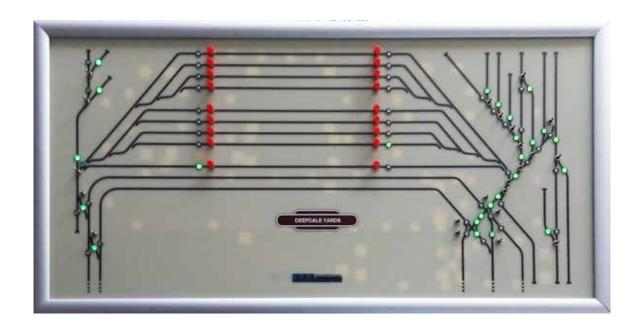
This control panel included a Super Panel, multiple Alpha Mimics, box size 5 and controlling 26 DCC accessory address. It also included route setting for the storage area via the Super Panel programming.
