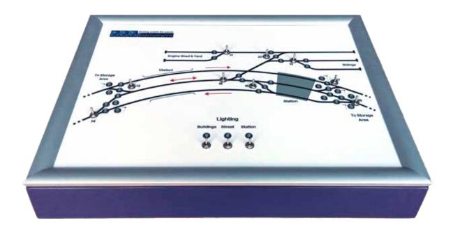
This control panel included an Alpha Encoder Unit, an Alpha Mimic, box size 3 and controlling 12 DCC accessory address.
