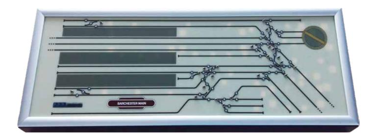
This control panel included a Super Panel, multiple Alpha Mimics, box size 4 and controlling 28 DCC accessory address.
