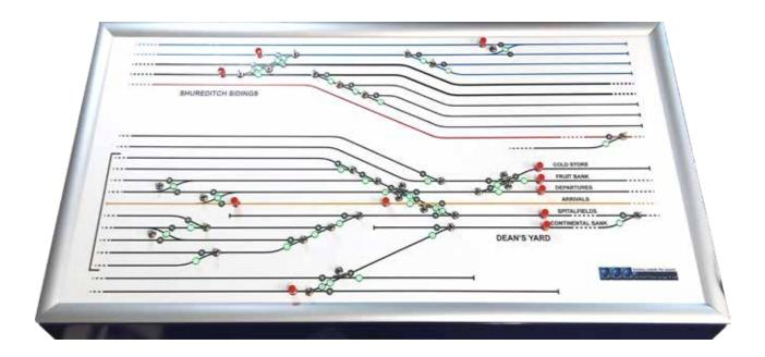
This control panel included multiple Alpha Encoder Units, Alpha Mimics, a custom connection plate, box size 5 and controlling 34 DCC accessory addresses.
